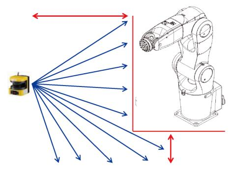
Figure 4.9 Laser scanner installation
