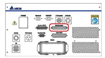
Figure 5.42 External encoder connector location
