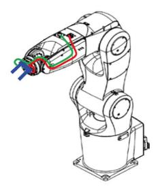
Figure 6.5 TCP Terminal air pipe and sensor wiring example
