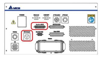
Figure 5.23 System .DIO and DC output connector locations
