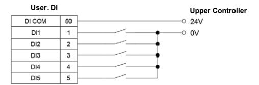
Figure 5.34 Input signal DI connected to the upper controller using NPN connection
