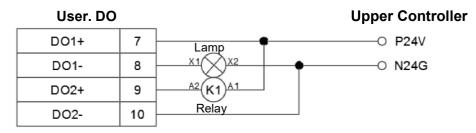
Figure 5.41 User. DO upper controller voltage mixed output wiring
