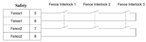
Figure 5.20 Wiring diagram for multiple safety protection devices
