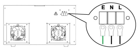
Figure 7.5 Quickstart wiring power wiring example
