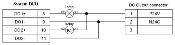
Figure 5.25 System DO DCV controller voltage output NPN wiring
