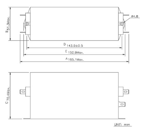
Figure 9.1 Delta wave filter 16DPCG5-1 dimensions
