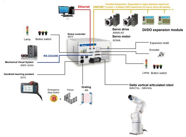
Figure 5.1 Controller peripheral system components
