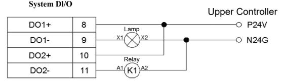
Figure 5.29 System DO upper controller voltage output PNP wiring
