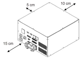
Figure 3.3 Controller installation spacing
