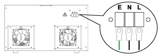
Figure 5.3 Power terminal wiring
