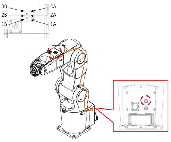
Figure 6.4 The robot's built-in internal air pipe location
