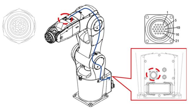
Figure 6.1 Internal wiring of the robot 12-Pos signal connector
