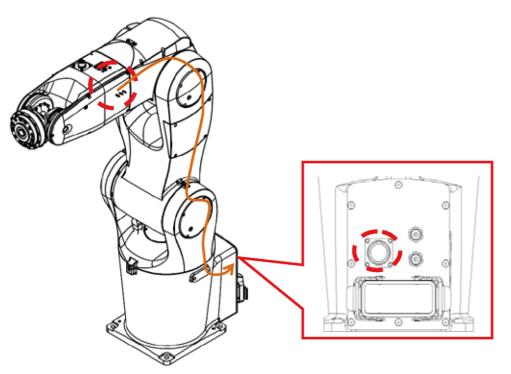
Figure 6.3 The robot's built-in solenoid valve wiring location
