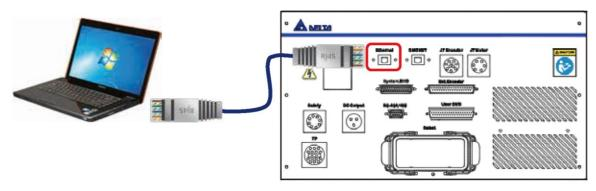
Figure 5.6 Ethernet connector location
