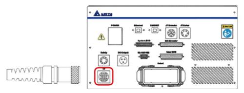
Figure 5.14 Handheld teaching pendant bypass connector location
