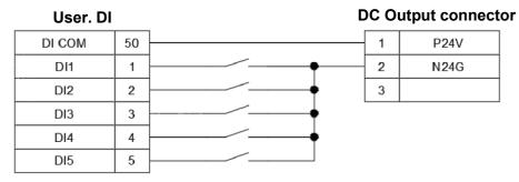
Figure 5.32 NPN wiring when the input signal DI uses power from the DCV controller
