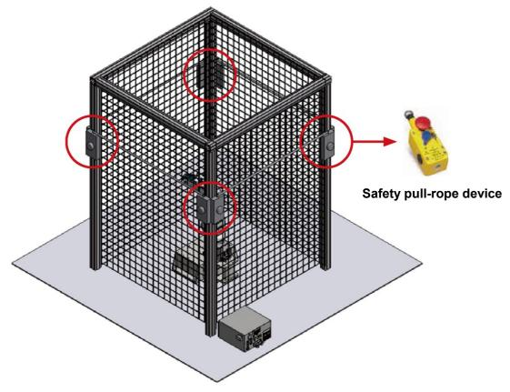
Figure 4.4 Safety pull-rope switch installation example
