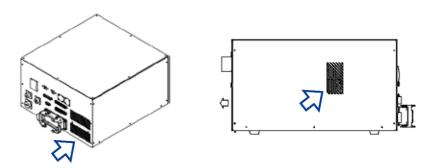
Figure 8.1 Controller ventilation filter locations
