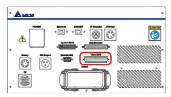
Figure 5.31 User. DIO connector location
