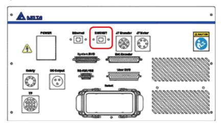
Figure 5.7 DMCNET connector location
