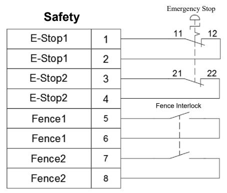
Figure 7.1 Emergency Stop button and safety signal wiring
