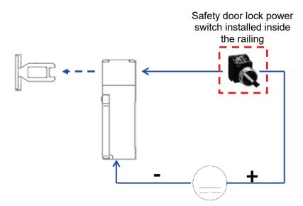
Figure 5.22 Electromagnetic safety switch wiring
