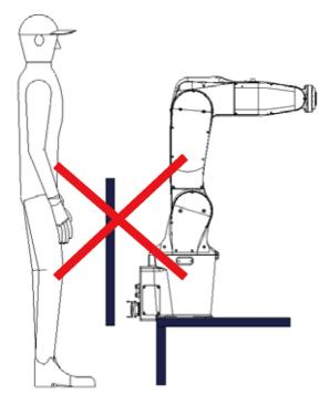
Figure 4.6 Insufficient railing installation height
