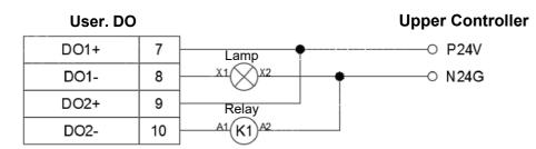
Figure 5.40 User. DO upper controller voltage output PNP wiring
