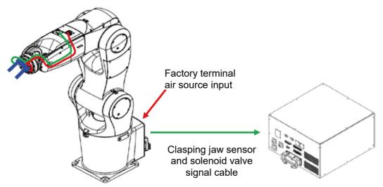
Figure 6.6 Robot clasping jaw signal and DCV controller connection
