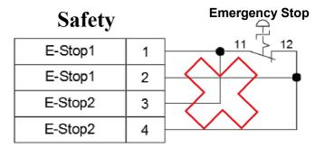
Figure 5.18 Incorrect wiring for a single NC emergency stop with the safety signal connected
