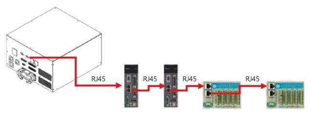
Figure 5.8 Multiple DMCNET connections
