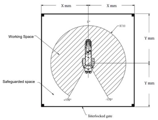
Figure 4.7 DRV70L safety grating installation distances
