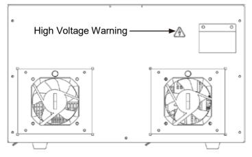
Figure 1.2 Sticker location on the back of the controller
