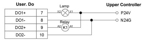
Figure 5.39 User. DO upper controller voltage output NPN wiring
