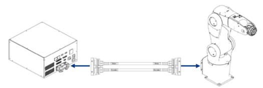
Figure 7.3 Robot and DCV controller cable connection
