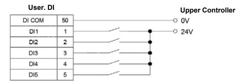
Figure 5.35 Input signal DI connected to the upper controller using PNP connection
