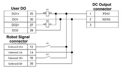
Figure 6.7 Wiring example for driving the solenoid valve
