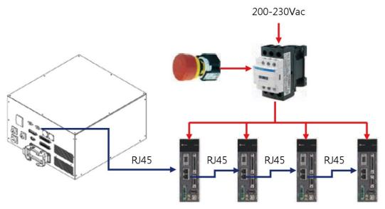
Figure 5.9 Controller with external servo drive system architecture
