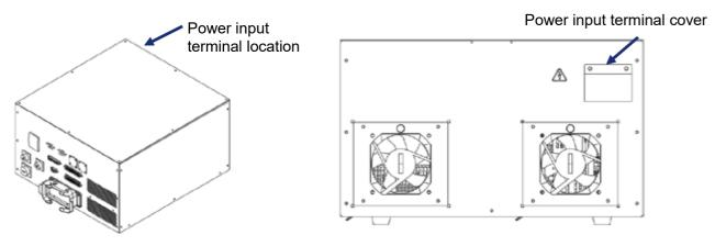
Figure 5.2 Power input terminal location
