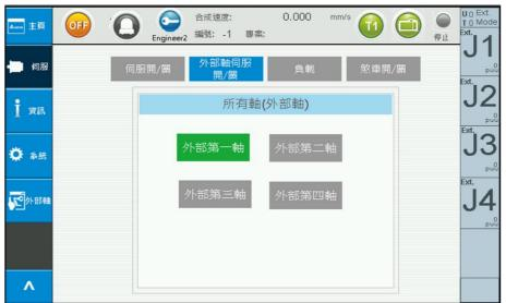
Figure 2-69 External Servo Switch - External First Axis Servo On
