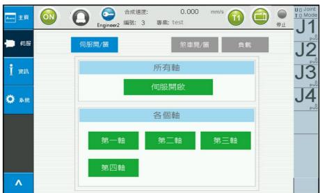
Figure 2-62 Servo Setting – All-axis Servo On
