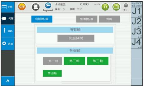
Figure 2-64 Servo Setting – First Axis Servo Off
