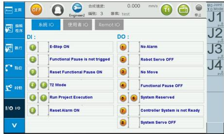
Figure 2-36 IO Surveillance - System IO
