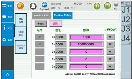
Figure 2-44 Modbus Information – Users Can Only Read the Modbus Address Information
