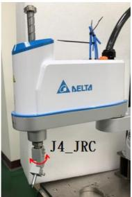
Figure 2-52 Illustration of the DRS Model Rotation Axis
