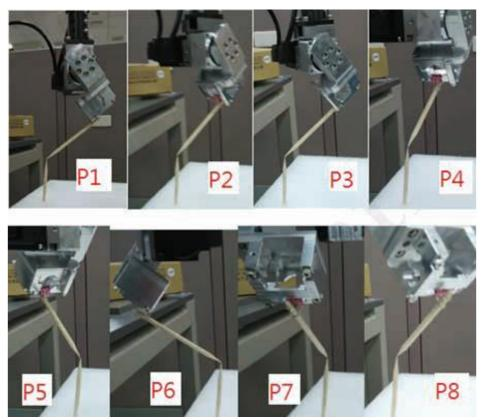
Figure 2-30 Point Information – Tool Size Calibration (Points P1-P8)
