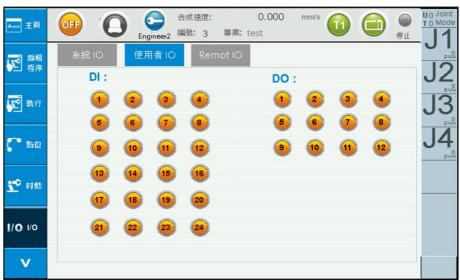
Figure 2-37 IO Surveillance - User IO
