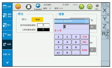
Figure 2-29 Select the tool frame ID with the points taught in the jog screen.
