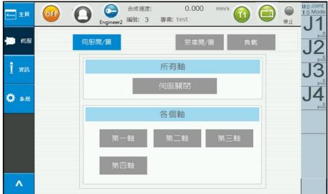
Figure 2-61 Servo Setting – All-axis Servo Off
