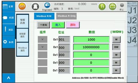
Figure 2-42 Modbus Information – Users Can Write Modbus Address Information Manually
