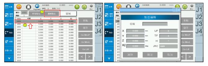
Figure 2-20 Point Information - Users Set the Local Point Parameters Manually
