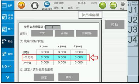
Figure 2-22 Point Information - User Coordinate +X direction Point Setting
