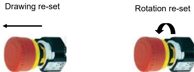
Figure3. 2 Emergency stop switch re-set method
